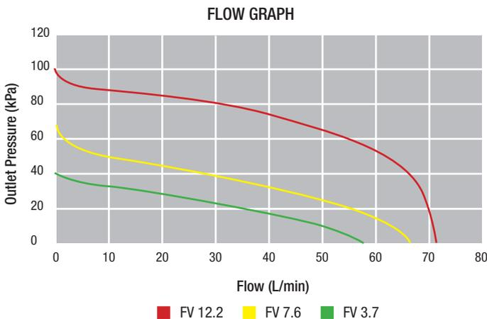
For increased flow rates or inlet pressure below 200 kPa, two valves in parallel may be required, doubling the flow.
