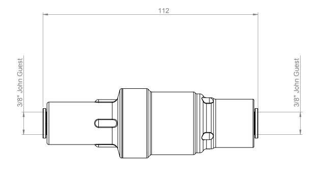
Filtamate pressure limiting valve FMP 3/8"
